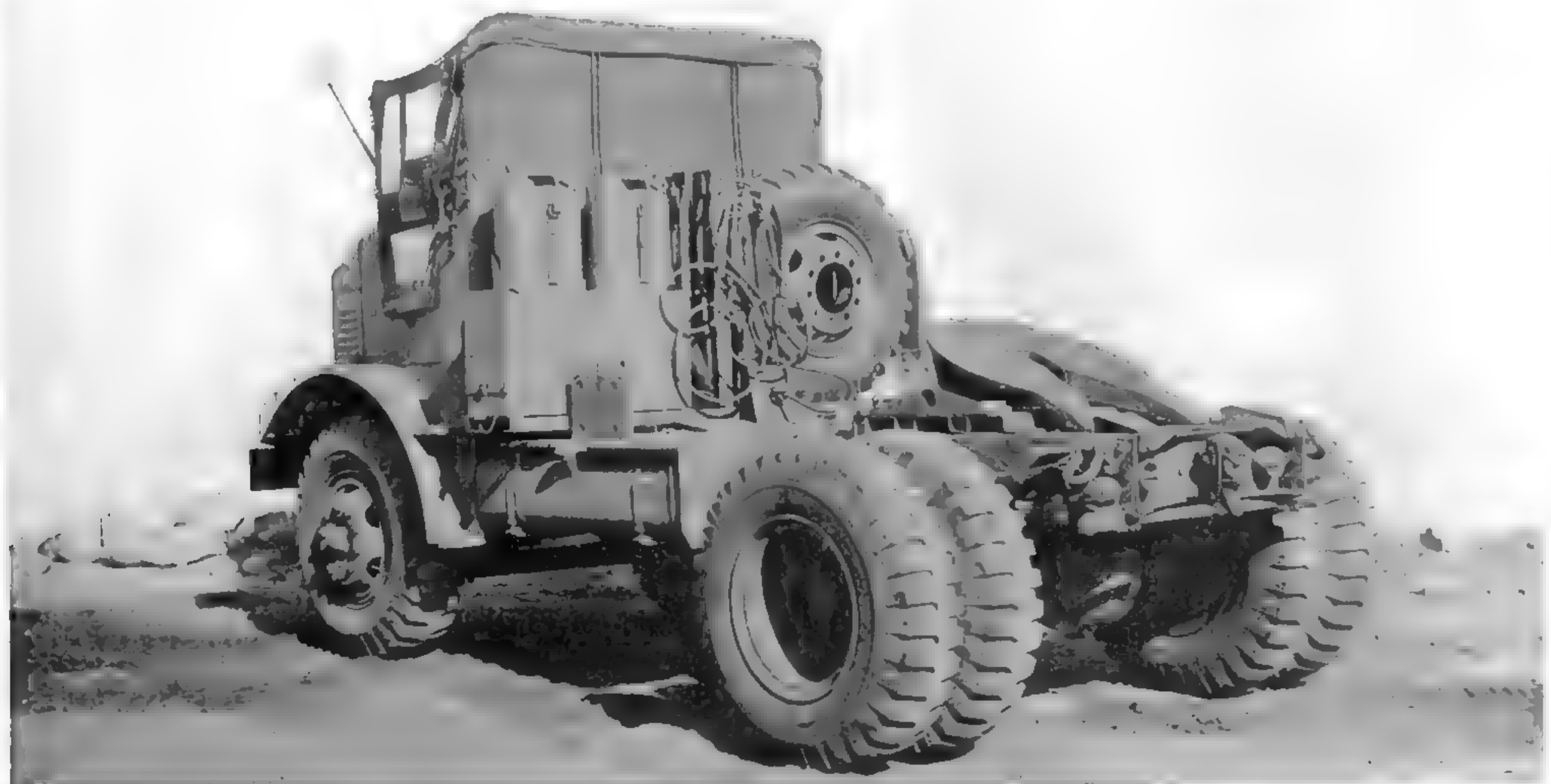
The M426 trailer air and electrical connections were mounted behind the cab, which was typical of tractor-trucks. Also visible is the vertically mounted pioneer tool rack, as well as liquid container racks and wheel chocks. (U. S. Army photo)
